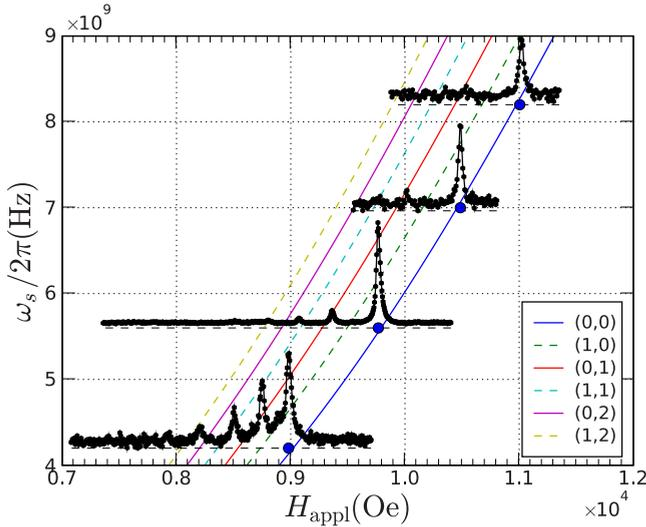
FIG. 9. (Color online) Mechanical-FMR spectra of the  $D_1 = 1.0 \mu\text{m}$  disk measured at 4.2, 5.6, 7.0, and 8.2 GHz and  $s \approx 3.1 \mu\text{m}$ . The blue circles indicate the positions of the most intense peak. The lines are the analytical predictions of the locus of the  $(\ell, m)$  modes when  $\theta_H = 4.9^\circ$  and  $H_{\text{off}} = -70 \text{ Oe}$ .
