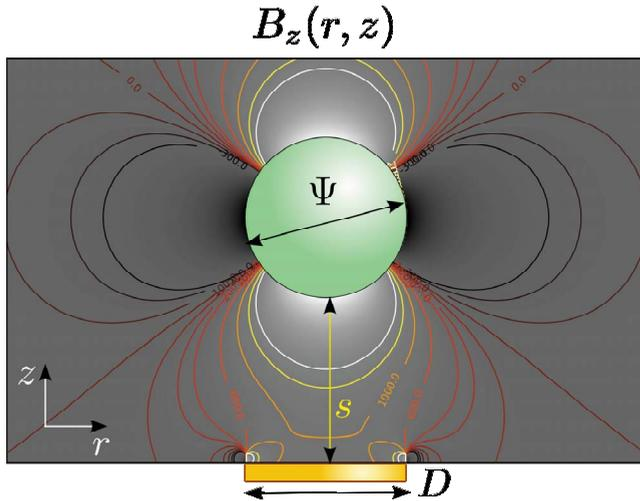
FIG. 3. (Color online) Visualization of the dipolar coupling interaction between a spherical magnetic probe (diameter  $\Psi$ ) and a cylindrical Py disk (diameter  $D$ ) separated by a distance  $s$ . The magnetic configurations in both objects are assumed to be saturated along  $z$ . The color lines represent the iso- $B_z$  field lines. The bright and dark shades separate, respectively, the positive and negative coupling regions.
