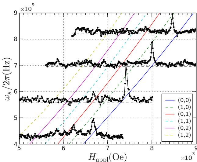
FIG. 10. (Color online) Mechanical-FMR spectra of the  $D_2 = 0.5 \mu\text{m}$  disk measured at 4.2, 5.6, 7.0, and 8.2 GHz and  $s \approx 1.0 \mu\text{m}$ . The lines are the analytical predictions of the locus of the  $(\ell, m)$  modes when  $\theta_H = 9.5^\circ$  and  $H_{\text{off}} = -760 \text{ Oe}$ .
