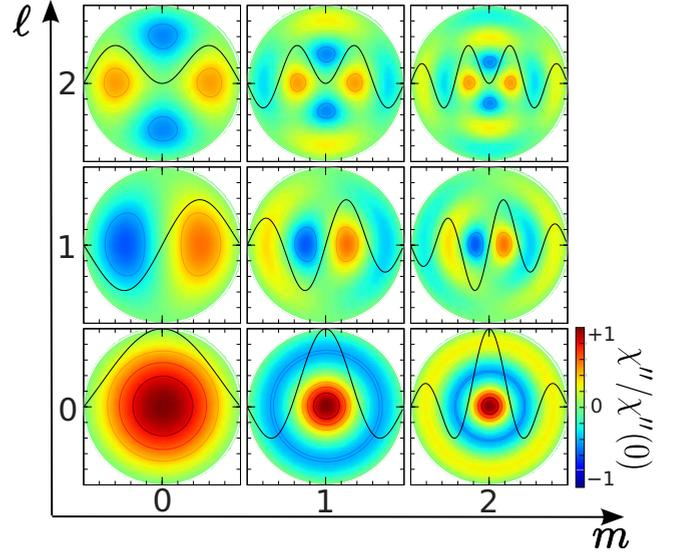
FIG. 6. (Color online) Color code representation of the eigenmodes basis  $\mathcal{J}_m^\ell(\mathbf{r})$ , where  $\ell$  and  $m$  indicate, respectively, the number of nodes in the circumferential and radial direction. Only the modes  $\ell=0$  couple to a uniform microwave excitation.
