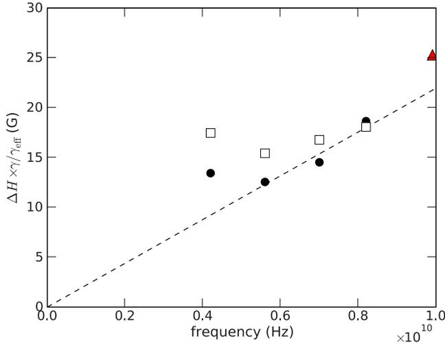
FIG. 18. (Color online) Frequency dependence of the linewidth measured on both the  $D_1=1.0 \mu\text{m}$  disk (full circles) and the  $D_2=0.5 \mu\text{m}$  disk (open boxes). The red triangle indicates the value measured by cavity FMR on the extended film on Si. The mechanical-FMR data are renormalized by  $\gamma_{\text{eff}}$ . The dashed line corresponds to a damping coefficient  $\alpha=6 \times 10^{-3}$ .
