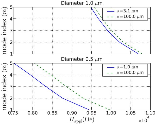
FIG. 7. (Color online) Calculated spectral deformation induced by the magnetic tip placed at distances  $s=3.1$  and  $1.0 \mu\text{m}$  above the disk samples  $D_1=1.0 \mu\text{m}$  and  $D_2=0.5 \mu\text{m}$ , respectively. The graphs show the downward shift in field of each resonance mode (indexed by  $m$ ) compared to the unperturbed FMR spectrum (dashed line).
