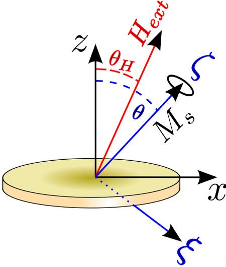
FIG. 11. (Color online) Graphic representation of the Cartesian frame  $(\xi, \zeta)$  (blue) rotated in the direction of the equilibrium magnetization when the applied field makes an angle  $\theta_H$  with the normal of the disk ( $z$  axis).
