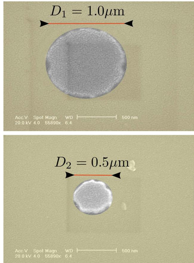
FIG. 8. (Color online) SEM images of the two Py disks samples. The images are being viewed at an angle of about  $15^\circ$  with respect to the normal of the substrate, thus distortions exist in the vertical direction.
