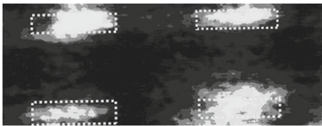
Fig. 6. The MRFM image is the image of a section of a microstrip array. The pumping frequency is 5.8 GHz, the bias field is 30 mT, and the distance between the probe and the sample is 1 \mu\text{m} . The dotted lines show the positions of the microstrips. The frame size is 11 \times 4 \mu\text{m} .
