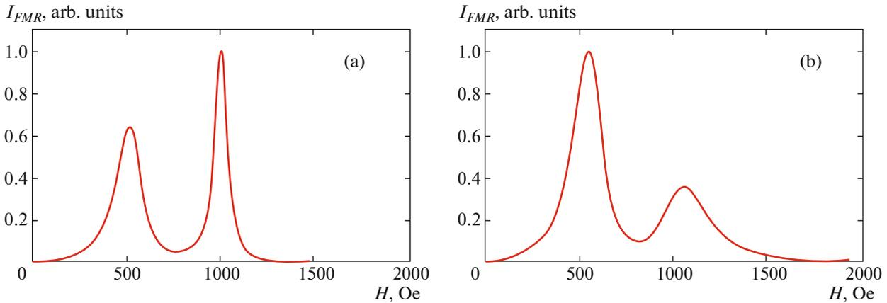
**Fig. 1.** (Color online) Dependences of microwave radiation absorption on the external magnetic field, recorded at room temperature for a structure with a weak ferromagnetic interlayer of thickness (a)  $d = 7$  nm and (b)  $d = 21$  nm.
