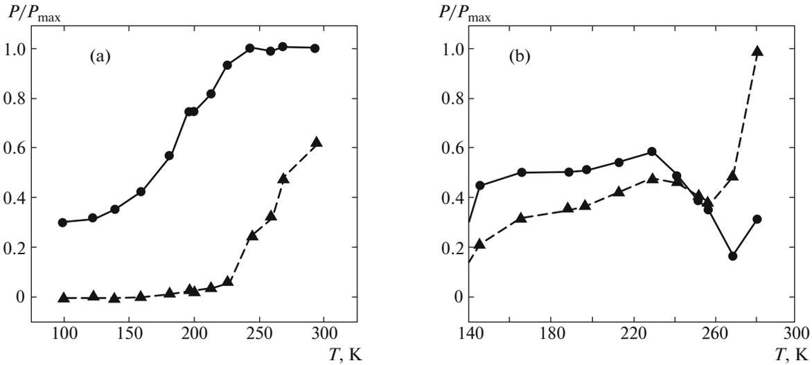
**Fig. 3.** Temperature dependences of the normalized amplitude of high-field (solid curves) and low-field (dashed curves) resonance peaks for a multilayer structure with interlayer thicknesses  $d = 7$  nm (a) and 21 nm (b).
