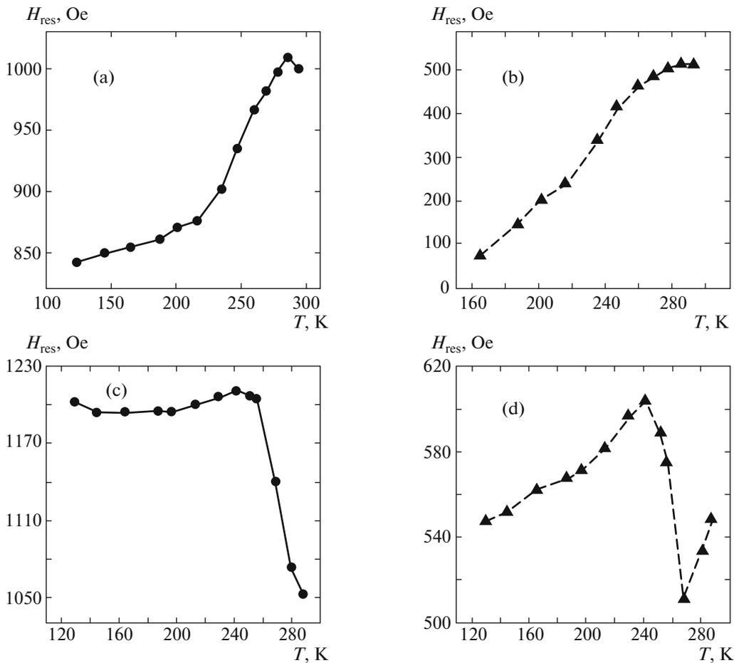
**Fig. 2.** Temperature dependences of resonance fields for (a, c) high-field and (b, d) low-field peaks for a multilayer structure with interlayer thickness  $d = 7$  nm (a, b) and 21 nm (c, d).
