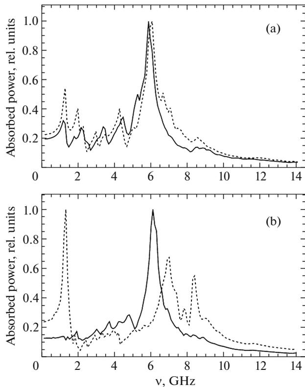
**Fig. 8.** Model spectra of system III for the configurations (a) H–H and (b) H–T. The solid and dashed lines represent the spectra obtained for alternating magnetic fields applied along the  $x$  and  $y$  axes, respectively.
