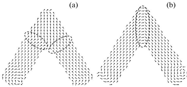
**Fig. 9.** Equilibrium magnetization distributions in system III for the configurations (a) H–H and (b) H–T.
