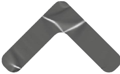
**Fig. 6.** Spatial distribution of the resonant magnetization oscillations (amplitudes of the  $z$ -component) in system II for the H–H configuration at the frequency  $\nu = 1.2$  GHz. The alternating magnetic field is applied along the  $x$  axis.
