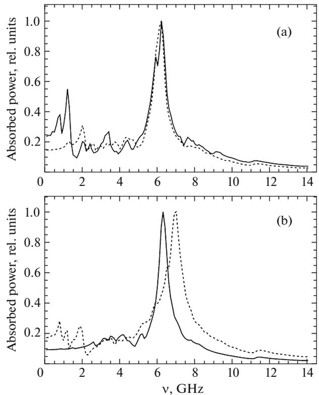
**Fig. 4.** Model spectra of system II for the configurations (a) H–H and (b) H–T. The solid and dashed lines represent the spectra obtained for alternating magnetic fields applied along the  $x$  and  $y$  axes, respectively.
