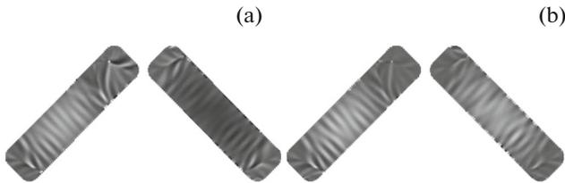
**Fig. 3.** Spatial distributions of the magnetization oscillations (amplitudes of the  $z$ -component) in system I for the H–H configuration: (a) quasi-optical mode and (b) quasi-acoustic mode.
