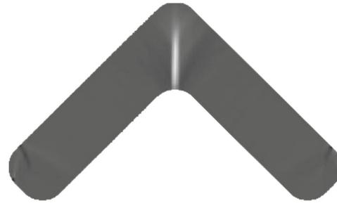
**Fig. 7.** Spatial distribution of the magnetization oscillations (amplitudes of the  $z$ -component) in system II for the H–T configuration at the frequency  $\nu = 1.9$  GHz. The alternating magnetic field was applied along the  $y$  axis.
