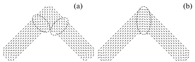
**Fig. 5.** Equilibrium magnetization distributions in system II for the configurations (a) H–H and (b) H–T. Ovals indicate regions of domain walls.
