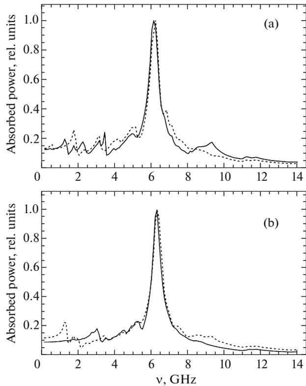
**Fig. 2.** Model spectra of system I for the configurations (a) H–H and (b) H–T. The solid and dashed lines represent the spectra obtained for alternating magnetic fields applied along the  $x$  and  $y$  axes, respectively.
