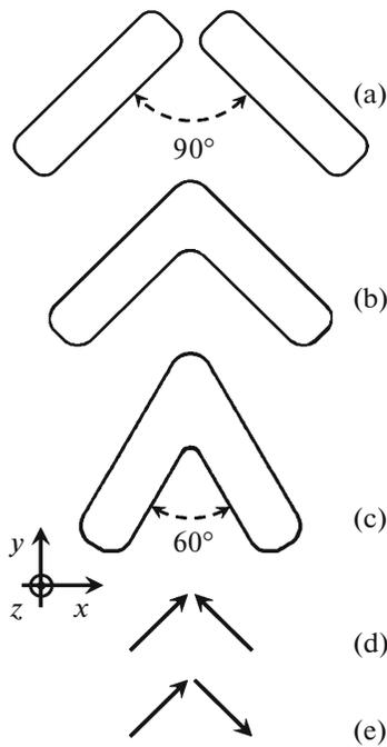
**Fig. 1.** Systems of interacting microstrip: (a) the system of individual microstrips tilted with respect to each other at an angle of  $90^\circ$  (system I), (b) the coupled microstrips tilted with respect to each other at an angle of  $90^\circ$  (system II), (c) the coupled microstrips tilted with respect to each other at an angle of  $60^\circ$  (system III), (d) the state of the magnetic moments of the microstrips H–H, and (e) the state of the magnetic moments of the microstrips H–T.
